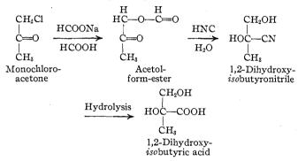
From 1204 g. of monochloro-acetone was obtained in seven runs, and after continuing fractionation until the fraction of desired boiling range no longer increased in weight, 524 g. of acetol-form-ester of boiling range  $166-169^{\circ}$  at atmospheric pressure; yield, 39.5%.
